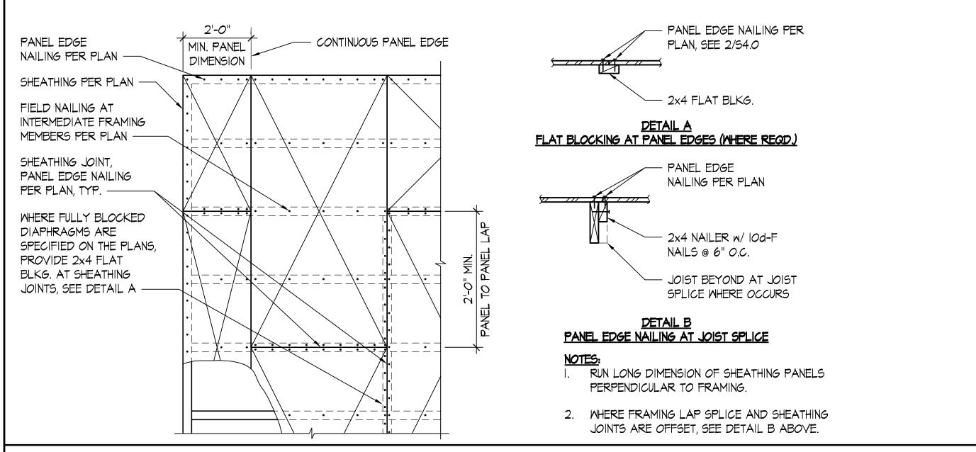
TYPICAL ROOF AND FLOOR DIAPHRAGM SHEATHING
